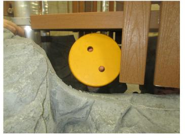
INSPECTION A Place torso template between post and rock. Template should be perpendicular to the opening. Torso template shall <u>not</u> pass between post and rock.
